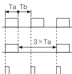
Therefore Ta(ON width) and Tb(OFF width) needed to be over min.signal width.
