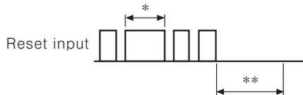
\*In case of a contact reset, it is reset perfectly if the ON time of reset signal is applied during min. 20ms even though chattering is occurred.
