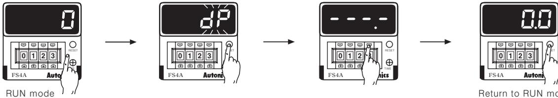
※Press RESET button for over 3sec., it advances to decimal point setting mode.
